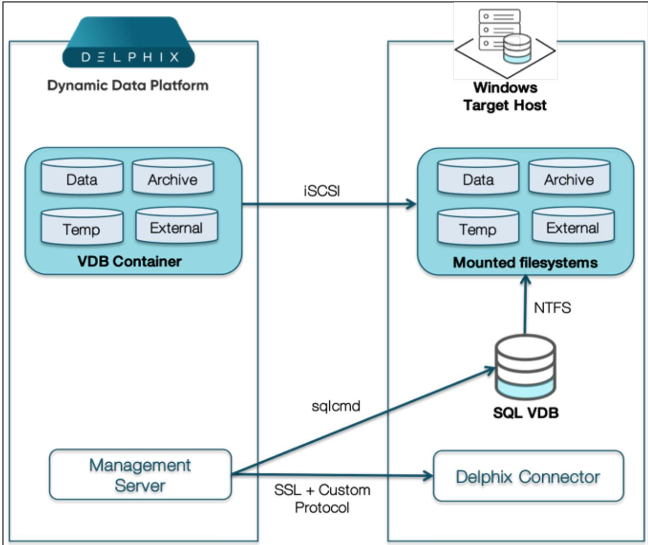
This block diagram shows how Delphix provisions VDBs to a Target Environment. The Delphix Engine (left) creates a set of virtual files from a snapshot that becomes the VDB container. These files are presented to the Target host (right) via iSCSI. Delphix calls the Delphix Connector on the Target and initiates the creation of a new database using the Virtual files. Once complete, the Virtual Database is brought online and made available for use.
